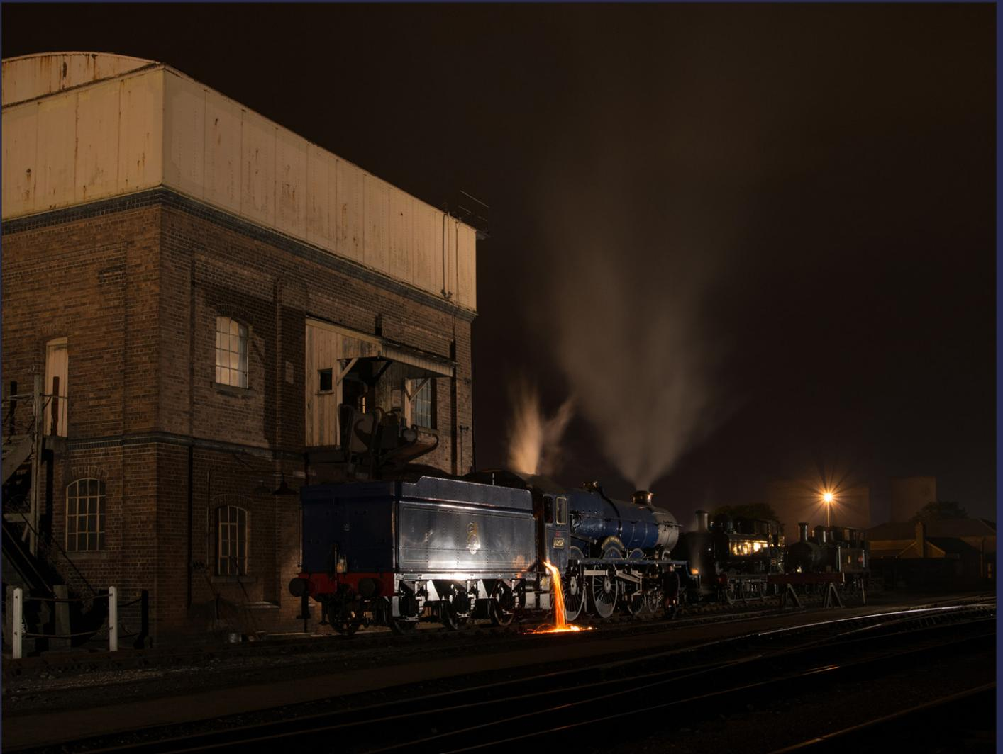
**Above:** It is the end of the working day and disposal duties take place on the last few locomotives still in steam. No. 6023 *King Edward II* has the clinker emptied from its firebox as preparations are made to add coal to the tender ready for the next turn. 8750 class 0-6-0PT Nos. 3738 and 1400 Class 0-4-2T No. 1466 await their turn on the ash pit. The evening was part of a Neil Cave photo charter on 29th June.
