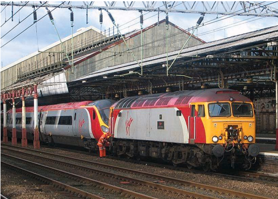
ABOVE: Having just arrived at Crewe on 13th February 2005, Class 57/3 No. 57305 John Tracy prepares to detach from 'Pendolino' No. 390026. The Class 390 will continue south to London Euston on electric power. A Non
